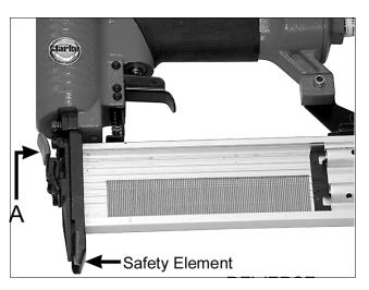
Turn on the air supply and check for air leaks. If any are apparent, rectify before proceeding. Ensure the operating pressure is set to between 4-7bar (60-100psi), depending upon the size of nail used and type of material being worked. The harder the material, and bigger the nail, the higher the pressure.
